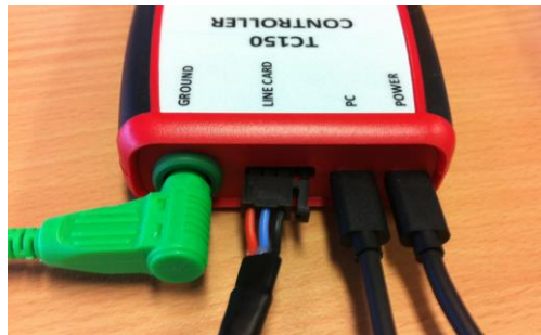
Fig 6 TC150 Tie Rite Controller connected to Ground, Line Card, PC/Laptop and Power (a battery)
