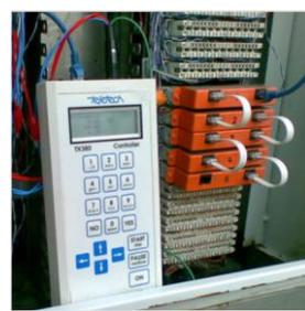
A TX380 tests and maps all the pairs connected via the multiplexers' shoes. Each TX380 is completely independent so several units can operate simultaneously on the same cabinet. This has significant accuracy and speed advantages.
